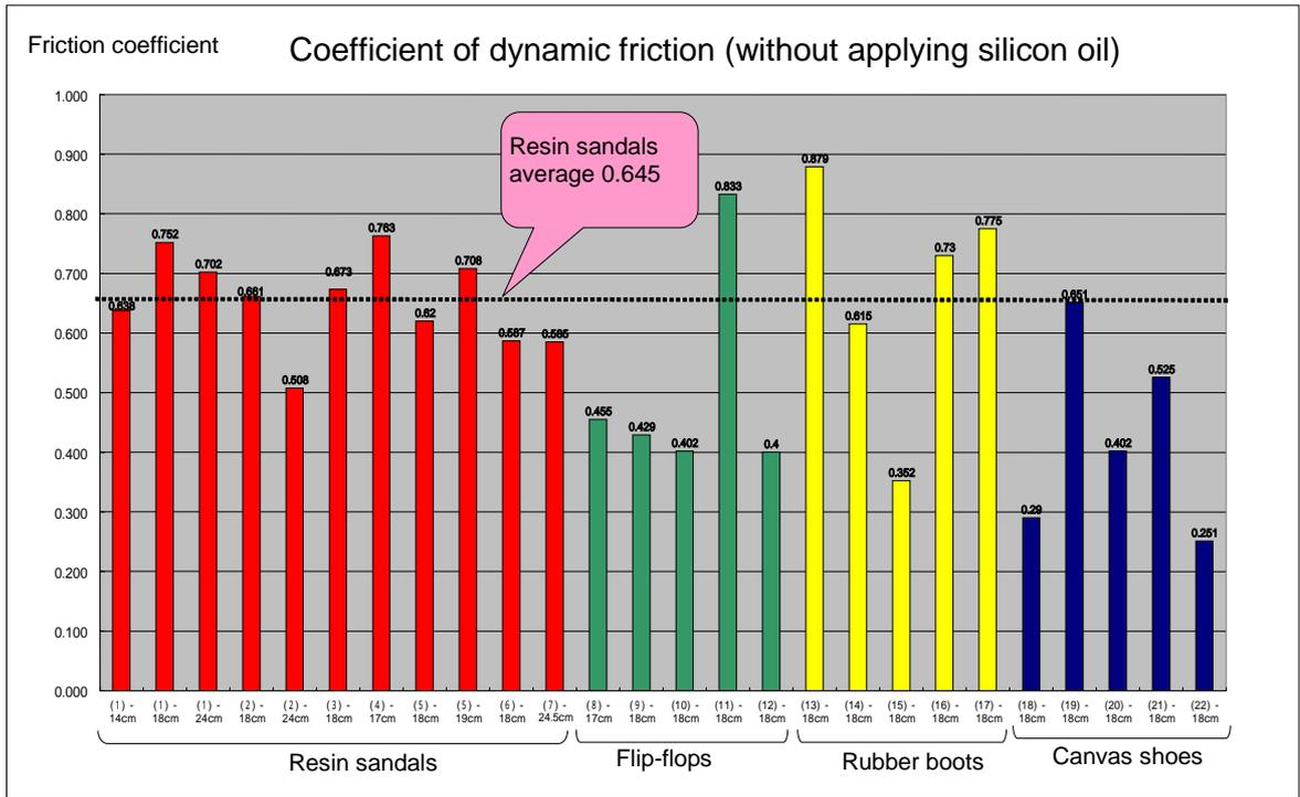
Figure 23: Comparison of dynamic friction
