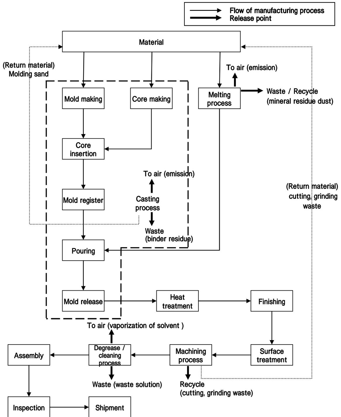
Figure 4. Stainless steel valve manufacturing process (casting)
