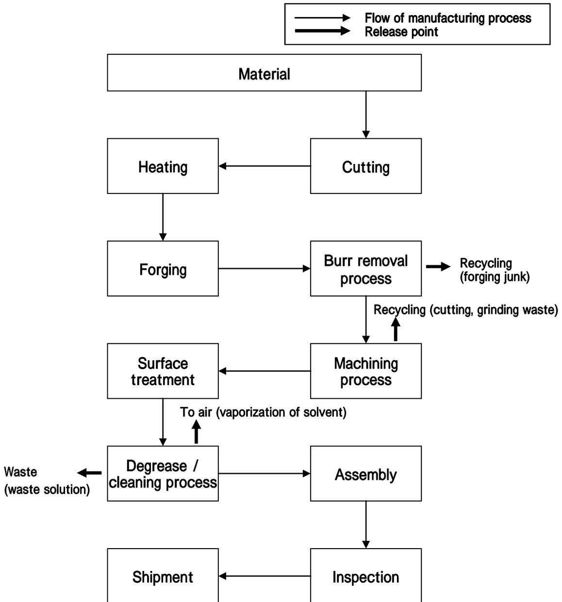
Figure 6. Forged valve manufacturing process
