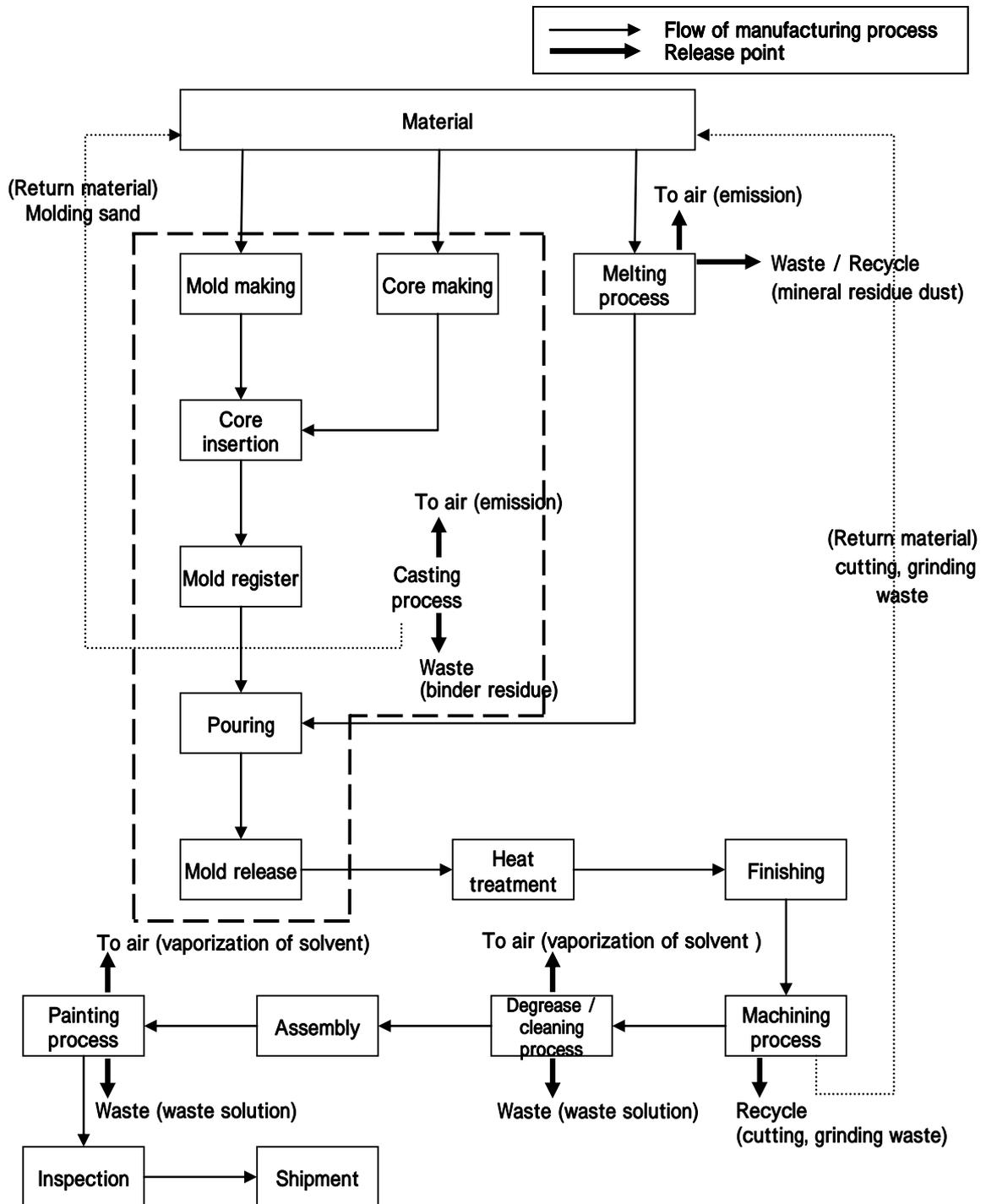
Figure 3. Steel casting valve manufacturing process
