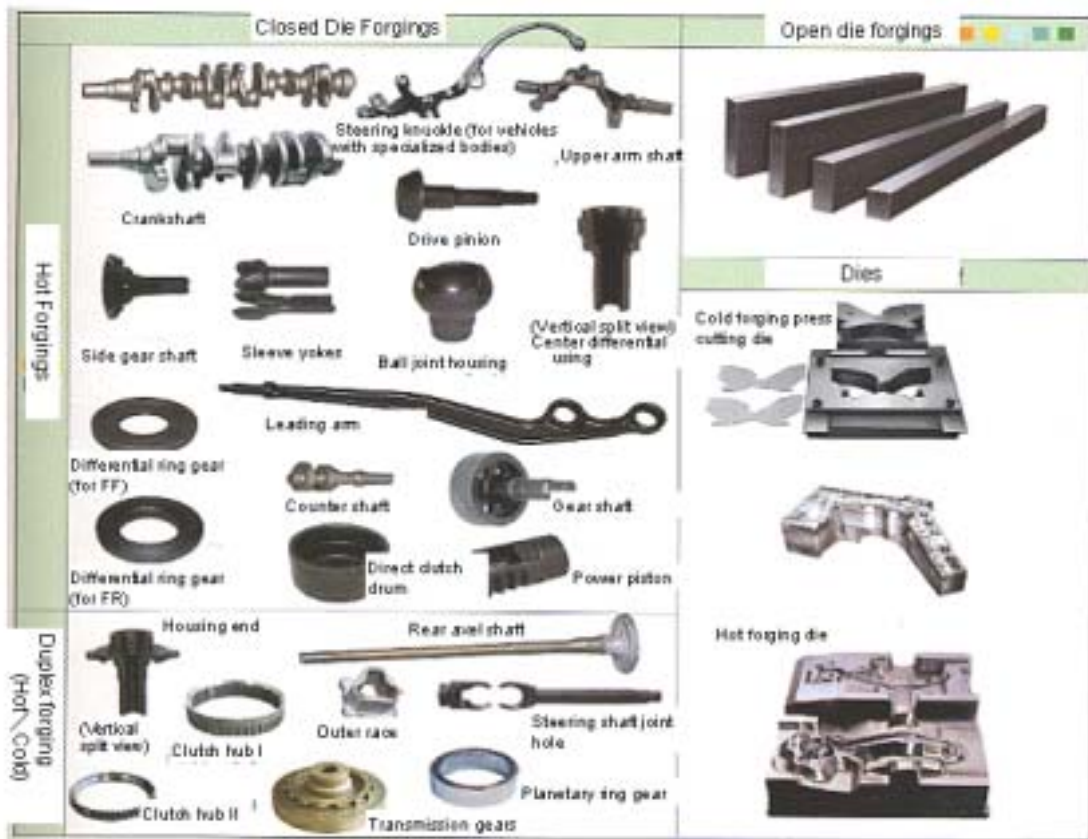
Figure 7 Examples of Major Products Manufactured in a Model Forging Plant
