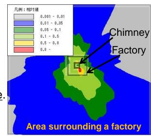
Example of atmospheric concentration distribution around a factory estimated with METI-LIS
